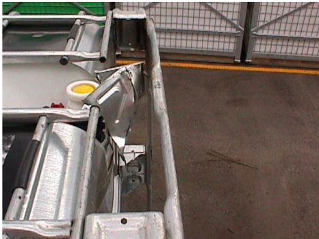
Pic 2: An example of a damaged pallet - Not acceptable
