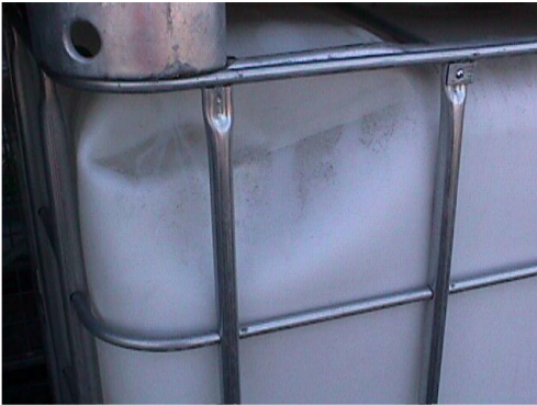
Pic 6: An example of a dented bladder - Not acceptable
