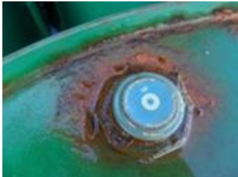
Pic 11: Rust on drum
