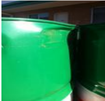
Pic 9: Drums that are not acceptable due to dents
