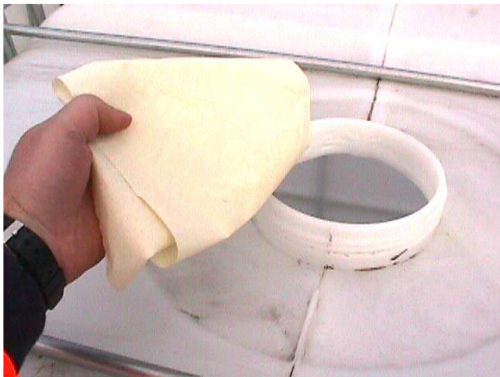
Pic 7: No visible discolouration on a clean paper towel when wiped against the inside surface
