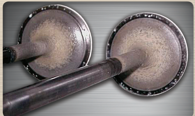
NOTICE EXHAUST VALVES AFTER 8,000 HOURS WITH DURATEC LFG
