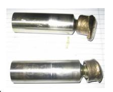
Parker axial piston pump failures at rolling mill automatic gauge control hydraulic system and related downtime were completely eliminated after change to Castrol Anvol SWX fire-resistant hydraulic fluid.
