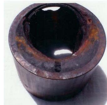
Bushing condition Previous Grease 8 weeks service
