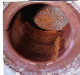
Bushing condition Braycote 2115-2 9 weeks service
