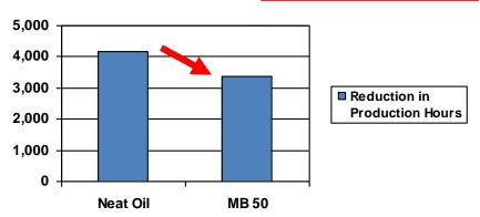
Hysol MB 50 has proven to be an extremely effective oil soluble coolant capable of replacing neat oil in the critical spline operation in the jet engine drive shafts. Castrol has been able to take these experiences and improve tool life and operator acceptance. These conversions have resulted in significant dollar savings and an enhanced work environment for the customer, as well as the elimination of chlorinated paraffins.
