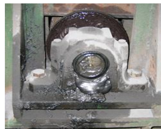
Previous grease would soften and run out of bearings & couplings due to the low centrifugal force resistance and poor roll stability.
