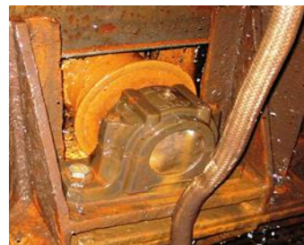
Previous grease completely washed out at furnace billet pusher due to low water resistance. Degraded grease caused bearing failure.
