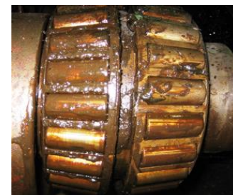
Previous grease completely washed out at furnace billet pusher due to low water resistance. Degraded grease caused bearing failure.
