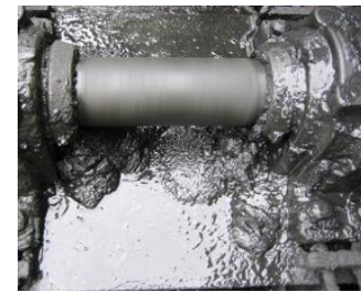
Previous grease would soften and run out of bearings & couplings due to the low centrifugal force resistance and poor roll stability.
