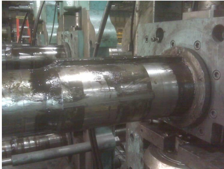
Typical roll shaft after disassembly, prior to conversion to Molub-Alloy 6040. Corrosion bands can be clearly seen across the shaft.
