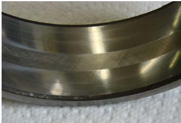
Minimal load zone area of bearing lubricated with Castrol Molub-Alloy 6282 Zinc-free grease.
