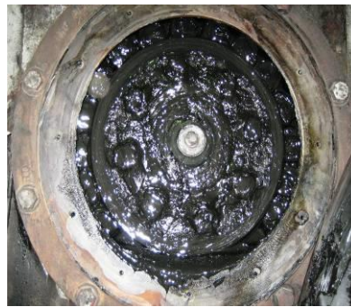
Bearings are sufficiently lubricated. Grease is not running out.
