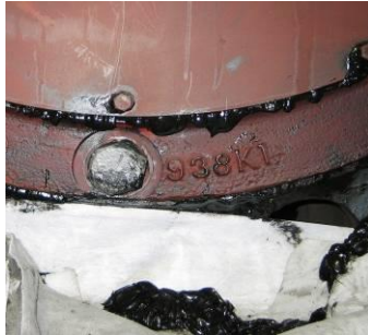
Grease appears too soft and running out of bearing.
