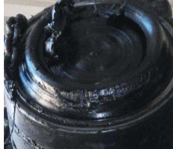
Grease is very hard like rubber material.
