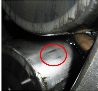
Fretting wear marks are present as shown in red.
