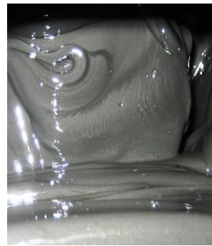
Grease appearance and consistency like new.
