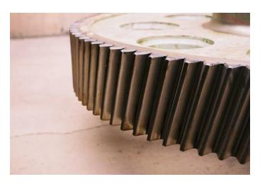
Ring gear from swing gearbox lubricated with Optigear 1100/1000 after 56,000 hours in service. Only 0.005" of wear measured.
