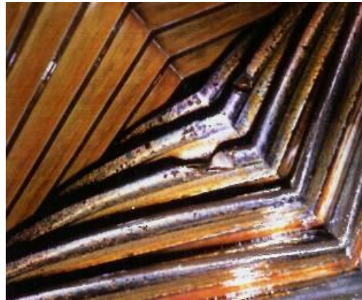
WCA Calendar Gearbox Condition prior to Castrol Heavy wear and missing teeth fragments
