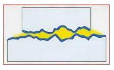
Step 1: Build up of load and pressure activates the additive combination to form a protective layer.
