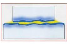
Step 3: At increasing loads, additives diffuse into the metal surface whereby the peaks flow into the valleys of the rough metal surface, creating a microsmoothening effect. This produces a very low coefficient of friction and spreads the gear load over a much larger surface area.
