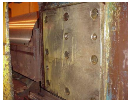
Roll liners with Castrol Performance Bio GR 8899
