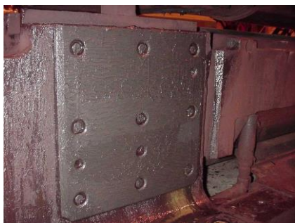
Roll liners with conventional lithium complex grease
