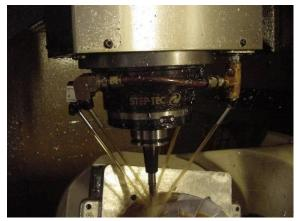
Application required 4 nozzles for cooling and chip evacuation
