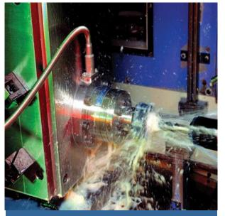
Castrol personnel worked closely with the customer to achieve significantly lower coolant costs through the use of a single coolant and equipment designed to remove coolant from the chips and recycle it for reuse back in the plant machines.
