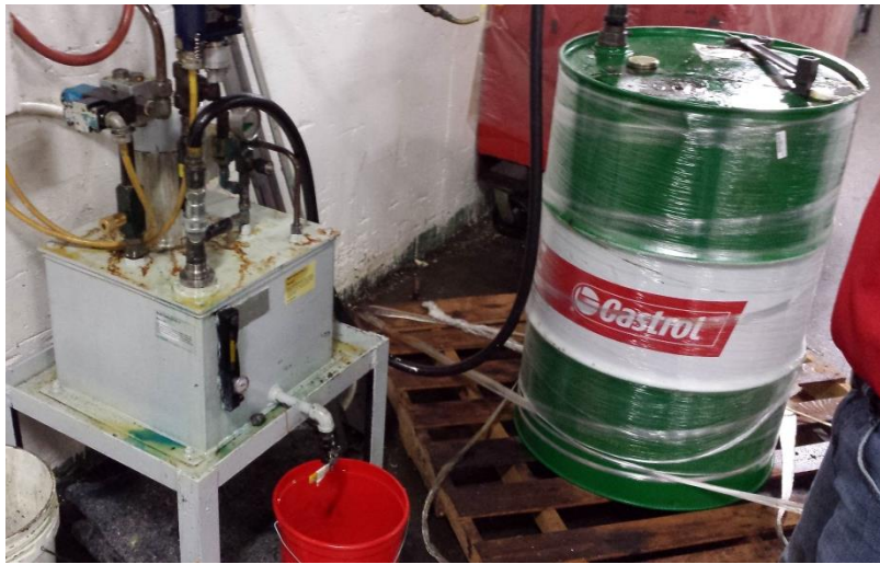
Slideway tank being filled with Tribol SW 1066
