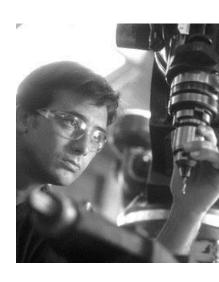
"...the surface appearance of the holes produced by the Castrol 334 at a high feed in bar stock have similar surface appearance to those produced previously by 50-50 at a lower drill feed rate."
