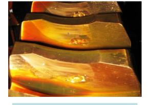
Cooling Bed South Drive - bronze wheel condition after 1 year in service before Optigear® Synthetic 800/2200 gear oil; note the sliding wear and spalling already forming
