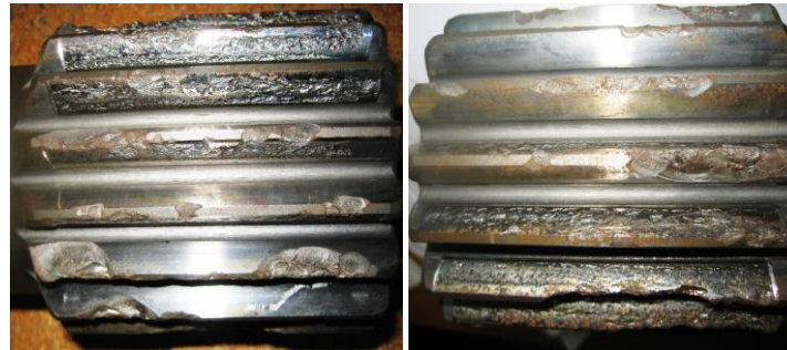
Connecting gear condition after only 2 years in service before Castrol Optigear 1100/1000 gear oil
