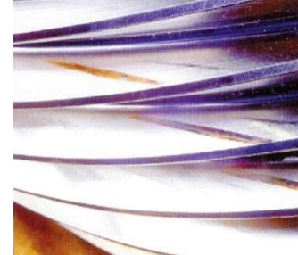
Unused gear with fretting wear
