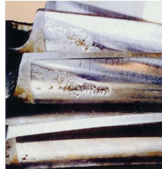
Significantly higher wear on one side of the gear is an indication of misalignment
