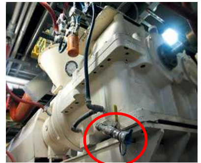
Quick-connect on gearbox for filter cart
