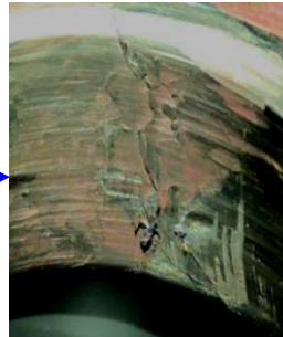
Fretting can occur on the inner ring of bearings where they meet the shaft
