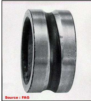
Typical wear pattern of bearing with misalignment. Bearing will have wider path or wear path running from one side of race to the other.
