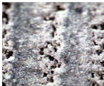
Current sparkover craters in the raceway of a bearing and on a gear surface
