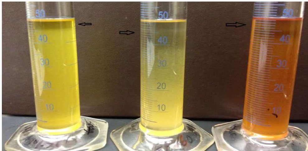
Photo showing haziness / separation in samples of gear oils mixed with VCI rust preventatives, indicating incompatibility
