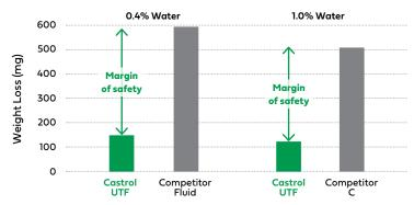
Wear and Corrosion in Contaminated Fluids
